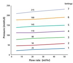
The valves perform within a tolerance range of the average pressure as shown here regardless of gravitational orientation:
