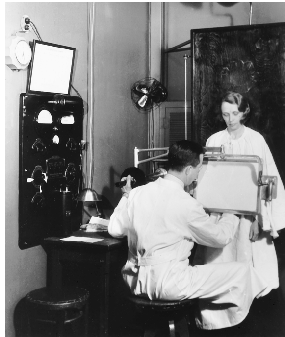
Figure 1. Photograph shows an early (1933) fluoroscopic system in use before the development of image intensification. An actual fluoroscopic examination with this device would have occurred in a darkened room. (Reprinted, with permission, from the Mayo Foundation.)
