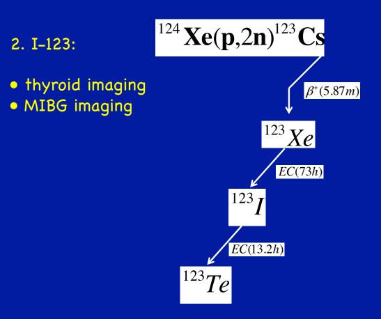
**Radionuclide Production: Cyclotron Produced**
