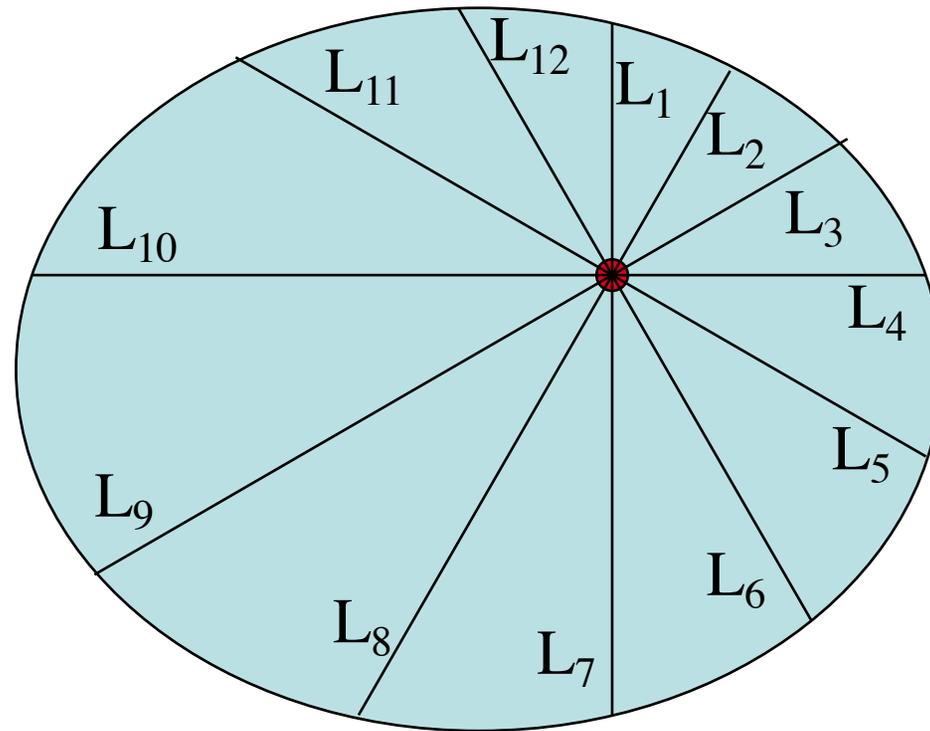
Attenuation Correction Factor:  $ACF(x, y) = \frac{1}{\frac{1}{N} \sum_{i=1}^N e^{-\mu L_i}}$
