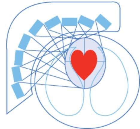
Pinhole collimation strategically positioned to focus on the "quality field of view"
