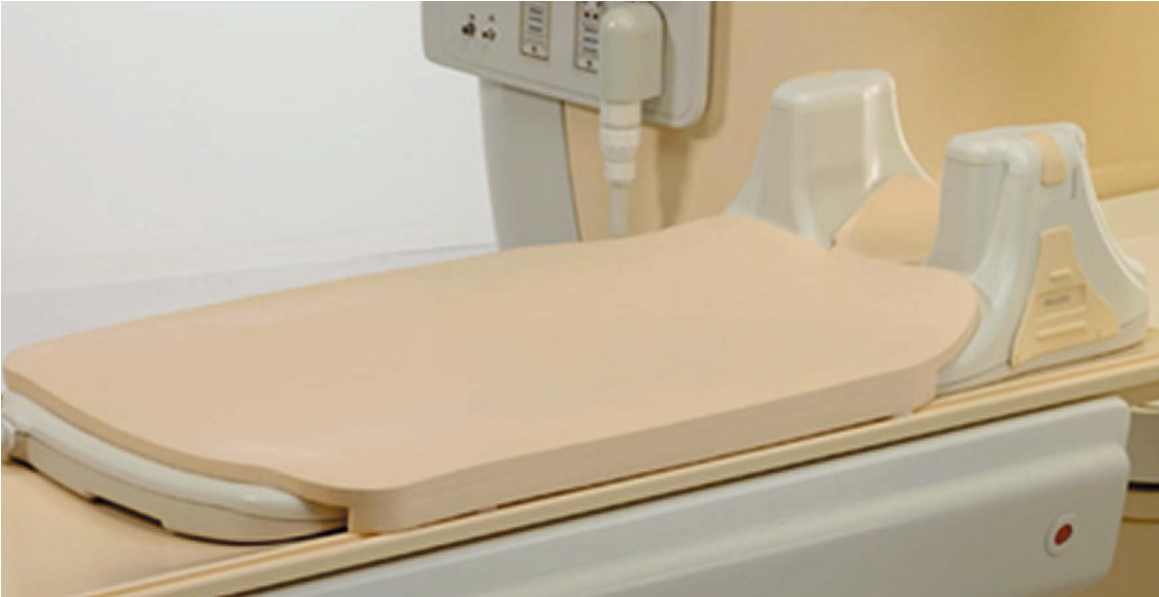
Figure 57.1 Spinal phased array coil.
